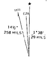
UTM GRID AND 1975 MAGNETIC NORTH DECLINATION AT CENTER OF SHEET
